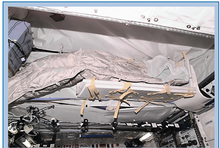
Temporary sleep station in the International Space Station, outfitted with polyethylene shielding and water to improve radiation shielding for astronauts. The thin flat panels are polyethylene shielding, while stowage water packaging is located above the sleep station.
